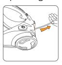
NOTE: Fully extend the power cord before each use. A yellow mark on the cord indicates the recommended cord length. Do not exceed the cord length beyond the yellow mark.
