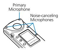
The noise cancellation features of the B3000 badge have been designed to provide significant improvement in speech recognition accuracy in environments with background noise compared to the older B2000 model.
