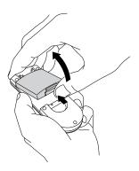
2. Insert the battery into the charger, and press down on the battery until you see the blue indicator light turn on.
