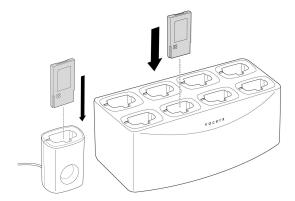
The green indicator light on the top of the charger will begin to blink when the battery is positioned correctly, and it will continue to blink while the battery is charging. When the indicator glows steadily, the battery is fully charged. Charging normally takes only a few hours.
