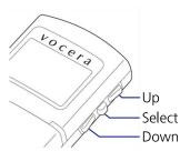
Use the Select button to choose a displayed item. To return to the main screen at any time, press and hold the Select button until the badge beeps. Pressing the Select button from the main screen takes you to the Messages screen.
