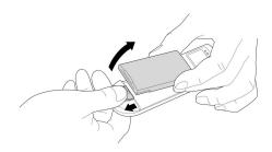
2. Insert the battery into the charger, making sure the battery label points toward the middle of the charger slot.
