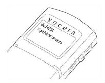
The B2000 badge automatically launches a screen saver when its display is inactive. The screen saver shows your first name and the first initial of your last name, along with an icon indicating the remaining battery life. The badge dismisses this screen saver immediately if the display needs to become active—for example, if you receive a call or a message.
