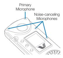
The noise cancellation features of the B3000n badge have been designed to provide significant improvement in speech recognition accuracy in environments with background noise compared to the older B2000 model.
