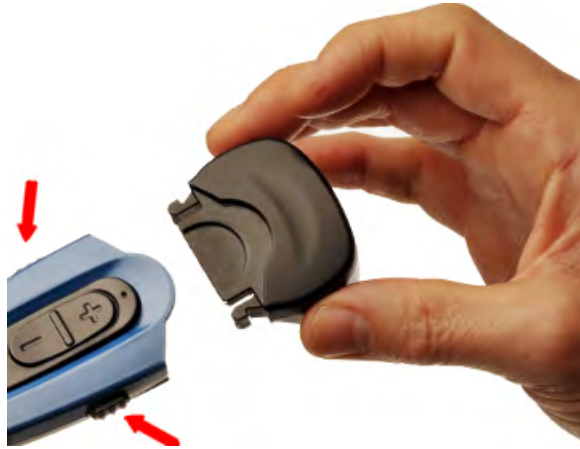
Figure 93: Battery Latches for Removing SRX2 Battery
