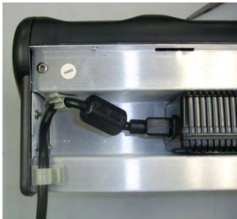
Figure 101: Cable Routed Through Plastic Clips
