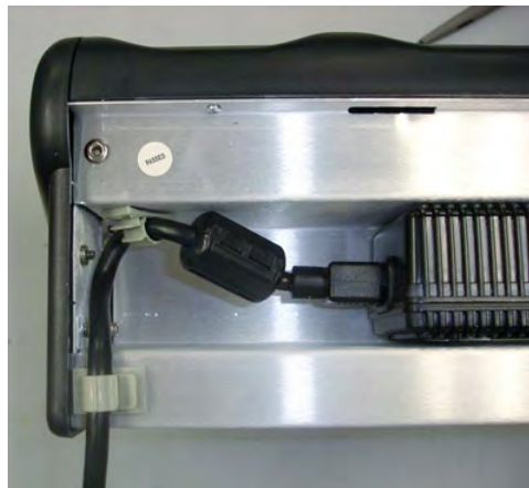
Figure 114: Cable Routed Through Plastic Clips
