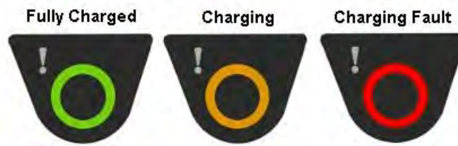
Figure 120: Battery Port Indicators
