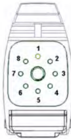
Figure 153: Vocollect Connector Pin Specifications
