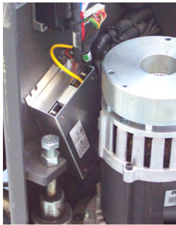
Figure 49: Power Supply Attached to a Secure Surface on the Vehicle
