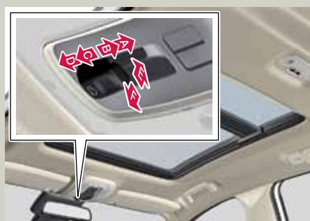
The first press on the control operates the sun shade; the second press operates the laminated panoramic roof. The sun shade must be fully open before the laminated panoramic roof can be opened manually. When the laminated panoramic roof is opened to the tilt (ventilation) position, the sun shade opens/closes automatically.
