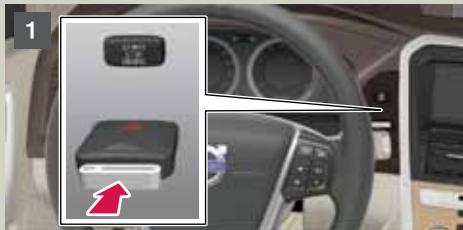
1. Holding the end of the remote key with the base of the key blade, insert the remote key into the ignition slot and press it in as far as possible.
