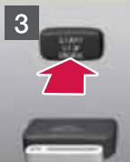
3. Press the **START/STOP ENGINE** button briefly to start the engine.
