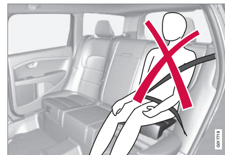
Incorrect seating position: the child's head is above the head restraint and the shoulder belt is not across the collarbone
