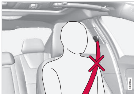
Incorrect height adjustment
