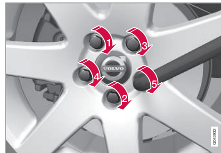
Tighten the wheel nuts
