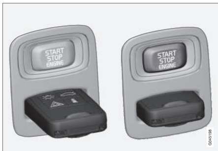
Ignition slot with remote key inserted (see Ignition modes (p. 80) for more information on ignition modes)
