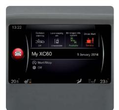
Many of the vehicle's functions can be controlled in **MY CAR**, such as setting the clock, storing the door mirrors' position, locks, etc.
