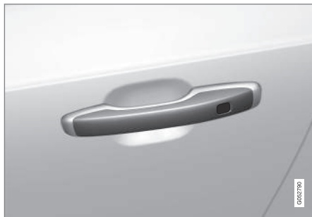
Outer indentation for locking, the pressure sensitive area on the inside of the handle is for unlocking
