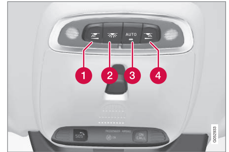
Controls in the ceiling console for front reading lights and courtesy lighting
