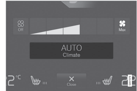
The Auto climate button in Climate view
