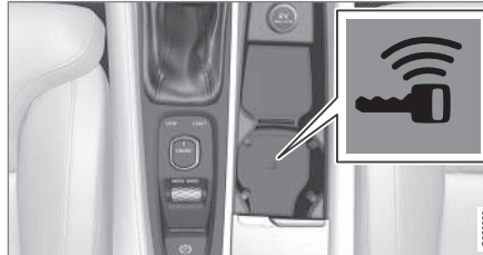
Back-up reader in the tunnel console
