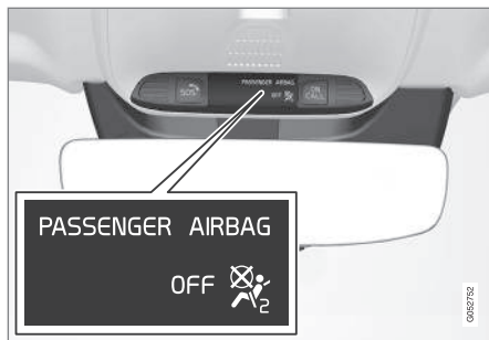
Occupant Weight Sensor (OWS) indicator light
