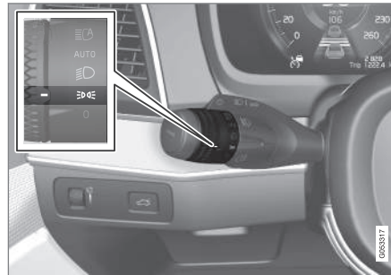
Lighting ring in the parking light position
