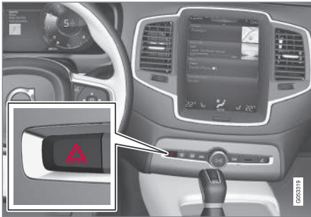
Hazard warning flasher button
