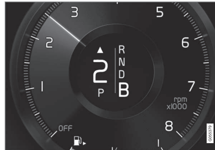
Gear shift indicator (generic illustration)
