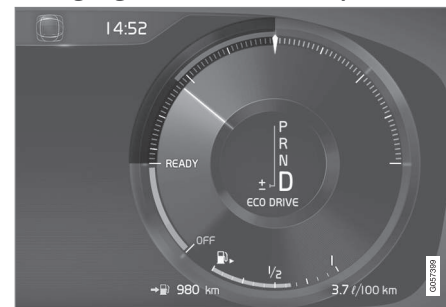
Eco gauge 12" instrument panel
