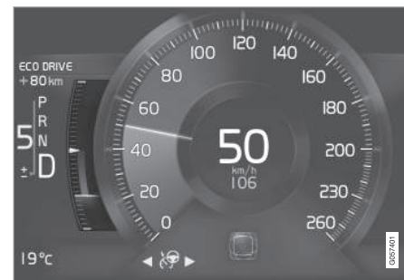
Eco gauge 8" instrument panel
