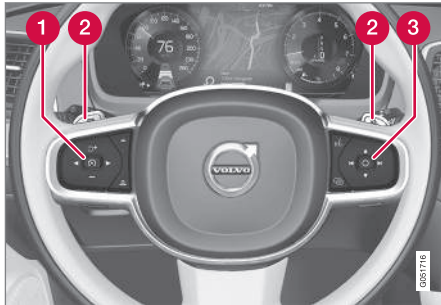
Steering wheel keypads and paddles*
