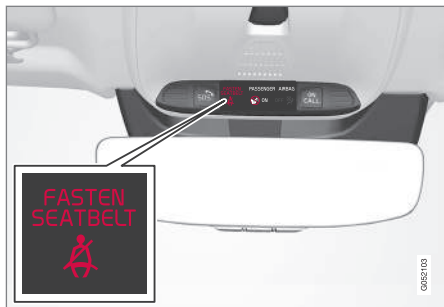
Seat belt reminder light in ceiling console
