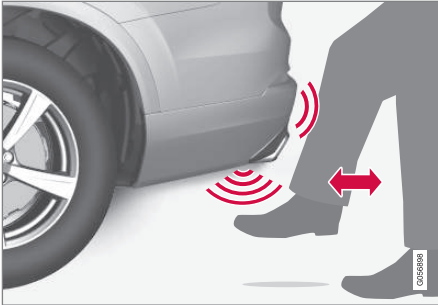
Kicking motion under the sensor's activation area
