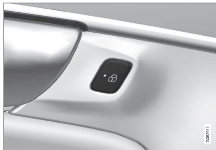
Lock button in a rear door
