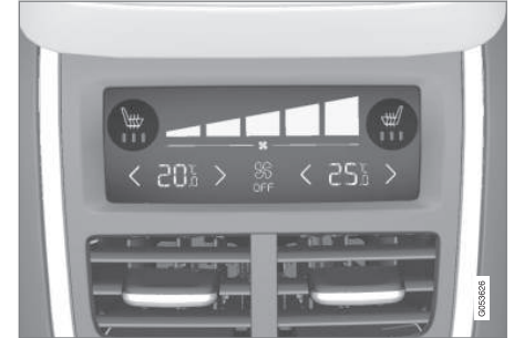
Seat heating indicator and control on the climate panel on the rear side of the tunnel console
