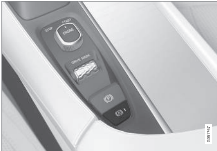
Auto-hold control and indicator light
