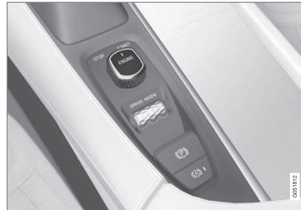
Start knob in the tunnel console
