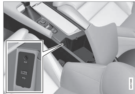
AUX/USB sockets in the tunnel console
