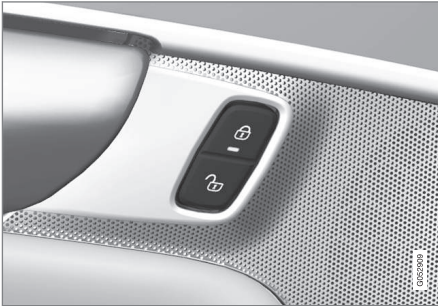
Front door lock buttons and indicator lights
