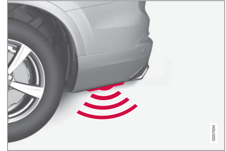
Sensor location on vehicles equipped with a skid plate/diffuser*
