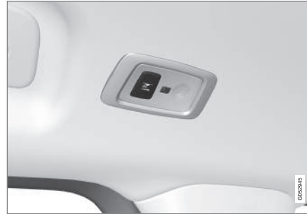
Rear reading lights: second row of seats
