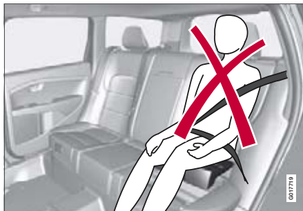
Incorrect position, the head must not be positioned above the head restraint and the seatbelt must not be below the shoulder.
