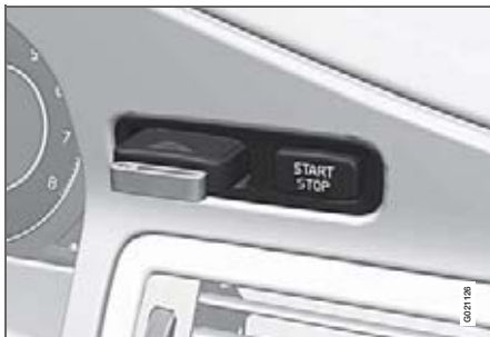
Ignition switch with remote control key, start and stop button (see more information on page 65).
