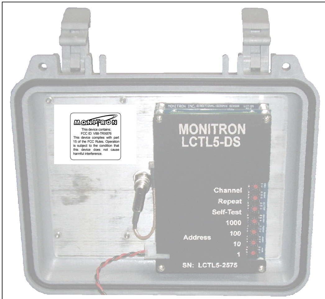
Location of FCC Label Inside LCTL5L-XX Lid (LCTL5 is shown for reference only)
