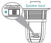
Press the **O** (Speaker On/Off) button on the back of the left speaker to turn it on.
