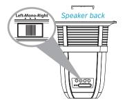
2 Press the **O** (Speaker On/Off) button on the back of the speaker to turn it on.
