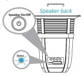
The **Status** light on the back of the speaker starts blinking blue, and the speaker says "Pairing."
