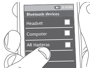
The speaker gives an audio signal when it's finished connecting to your smartphone. The indicator light on the top of the speaker turns solid blue.
