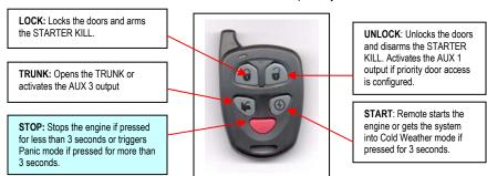
N.B.: Pressing the LOCK and UNLOCK buttons simultaneously will activate the AUX 2 output.
