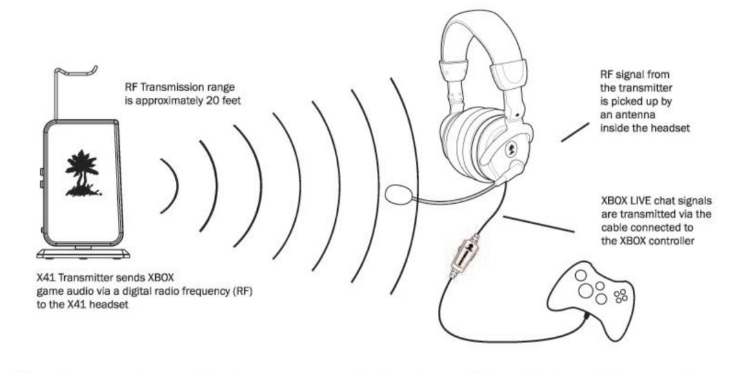
When the transmitter and headset are communicating, the top LED on the front of the transmitter will be on. If this LED is slowly pulsing, it means the transmitter can't communicate with the headset. This could happen if the headset is turned off, out of range or needs to be "paired".
