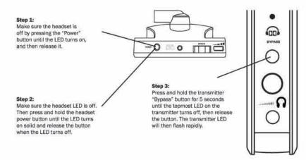
After a few seconds, the topmost transmitter LED should be on solid and the headset LED should be flashing about once per second, indicating that the units are paired.
