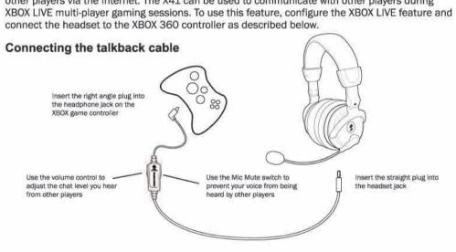
Mic Mute Switch: The mute switch on the talkback cable can be used to silence the headset mic
