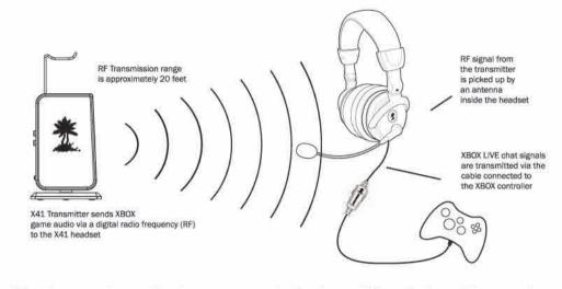
When the transmitter and headset are communicating, the top LED on the front of the transmitter will be on. If this LED is slowly pulsing, it means the transmitter can't communicate with the headset. This could happen if the headset is turned off, out of range or needs to be "paired".
