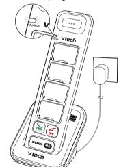
You hear a confirmation tone when the registration process completes. It takes up to 60 seconds to complete the registration. If registration fails, you hear an error tone, and the **CHARGE** light alternates red and green slowly when it is taken out of the cradle. Start again from Step 1 above.
