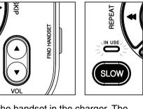
2. Put the handset in the charger. The handset **CHARGE** light alternates red and green quickly to indicate the registration is in progress.
