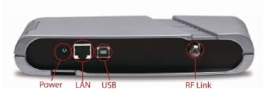
Figure 3 – V284 WMU rear Panel Ports
