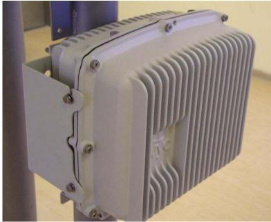
5. Assemble GND wire with Ring terminal on the grounding screw (see the screw size in balloon 9of the table in section 2) that placed on the V290.
