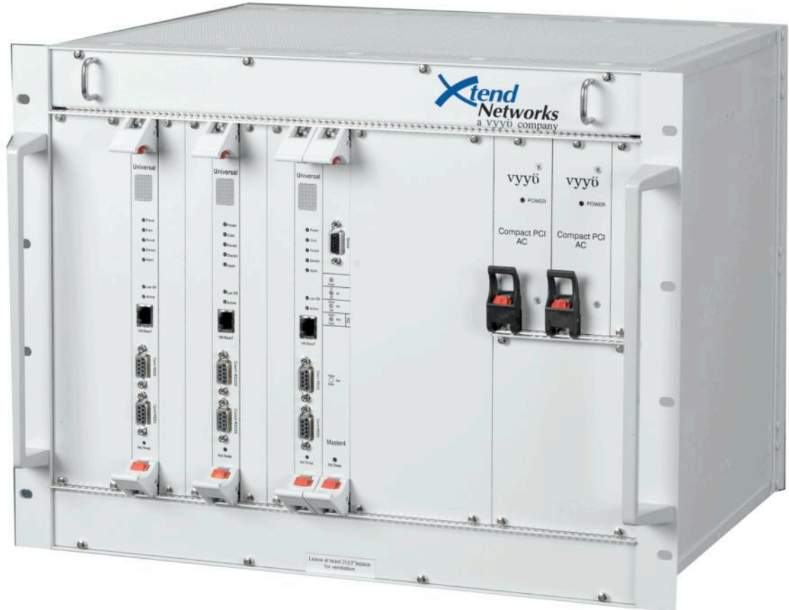
Figure 1-1. The WMTS Chassis with (from left to right) Upstream card, Downstream card, Control and Forward card, MASTER4 card, and Power Supplies shown.
