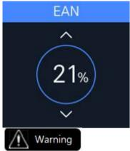
Nitrox can be set up at EAN in setting menu before diving.
