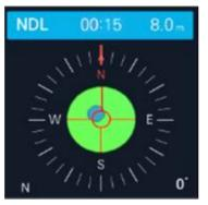
□ This device will automatically switch to diving mode when it reaches over 0.5m of depth.
