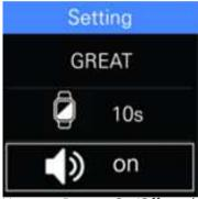
You set Buzzer On/Off, and as the results, all buzzers include alert in diving mode and others can be turned off. It will help you to manage battery.
