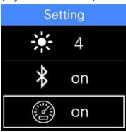
If it is set as gauge mode before start diving, it will automatically enter gauge mode, and warning phrase and buzzer will not ring, as well algorithm also won't be applied.
