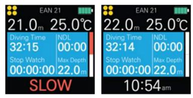
Do not exceed the maximum speed for ascend(9m/min). Danger of exceeding the maximum speed is to cause serious injuries or deadly situation.
