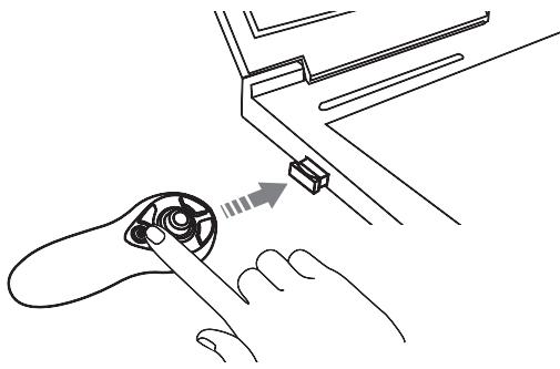
Notes: The Receiver is very small and can remain plugged into your computer. If you decide to remove the Receiver, store it inside the Battery compartment.
