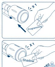
2 To delete existing user card: Programming Card x 1 time, existing user card x 1 time for 5 seconds.
