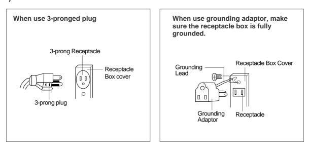
"THE CANADIAN ELECTRICAL CODE DOES NOT ALLOW THE USE OF THE GROUNDING ADAPTOR"
