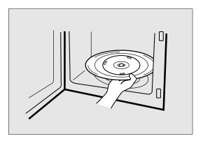
7 The roller guide and oven cavity floor should be cleaned regularly to avoid excessive noise.
