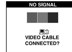
No Signal screen is displayed when the D-Sub signal connector is not connected or the status of the monitor is on DPMS mode.
