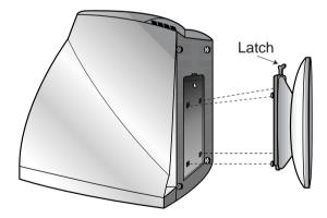
If you want to remove the tilt/swivel stand on the monitor, press the latch and pull the tilt/swivel stand toward the back of the monitor. Lift the stand to separate.
