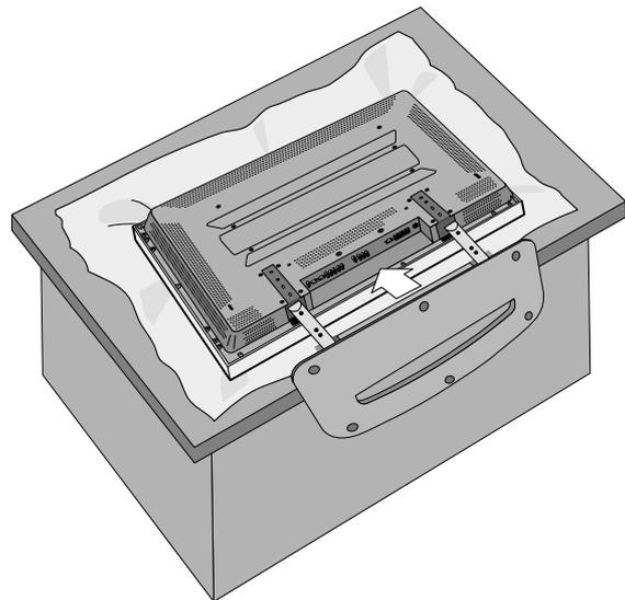
**3** Engage the assembled stand with 6 screws (M6) enclosed.
