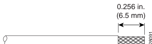
Figure 44 Stripping the Cable Jacket
