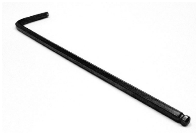
Figure: 7-8 Tool to screw off the screw of reset button.
