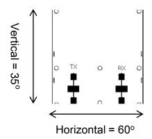
Antenna consist of 2 parts; Tx and rx. They are same1x3 patch type having 60 degree horizontal half-power beam width and 35 degree vertical half-power beam width.
