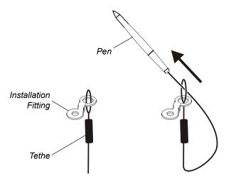
3. Attach the installation fitting to the back of the interactive pen display using a screwdriver or a small coin.
