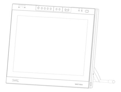
The ID422w interactive pen display is a 22" (58.1 cm) Liquid Crystal Display (LCD) interactive screen that acts as an input and output device.
