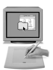
Pointing and selecting. Move the Intuos2 Pen above the tablet surface to position the screen cursor, then press the pen tip on the tablet to make a selection.
