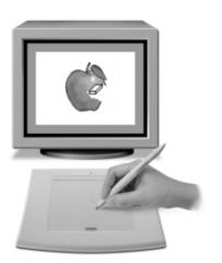
Erasing. In supporting applications, the pen's eraser works like the eraser on a pencil. In text applications, use the eraser to select text, then lift the eraser from the tablet to delete the text.
