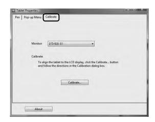
**3** Click again in the middle of the cross mark that is now in the bottom right-hand corner of the screen while sitting in your normal seating position and the cross mark will disappear. The process of synchronizing positions is now complete.
