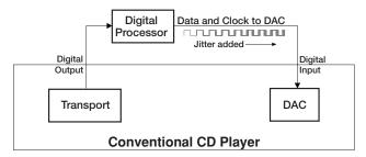
Using ClockLink with an external processor, the Wadia 861 ignores the incoming clock and uses the master oscillator at the DAC. As a result, jitter added by the external digital processor does not affect sonic performance.
