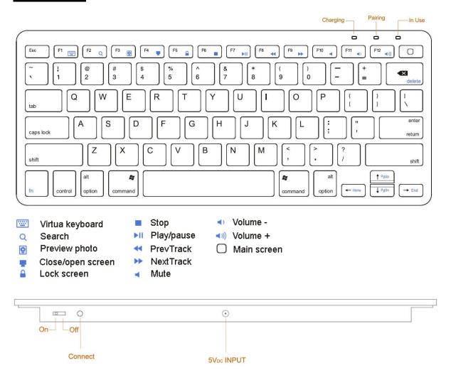
Red LED Blinking: Pairing or Low in Battery
