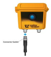
2 Tighten connector enough to slightly compress connector gasket.
