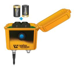
3 Immediately upon installation of 2nd battery, the blue LED on the front of battery-powered node will quickly give three (3) "blinks". This means the unit is in standby mode and ready to be powered up.
