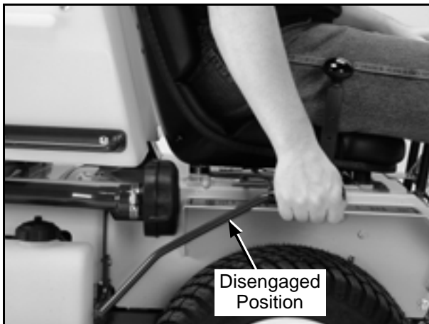
Blade Clutch Disengaged
