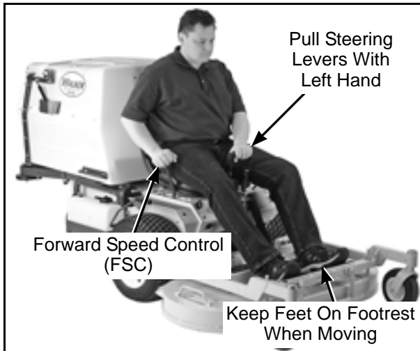
Correct Operator Hand Position on the Controls
