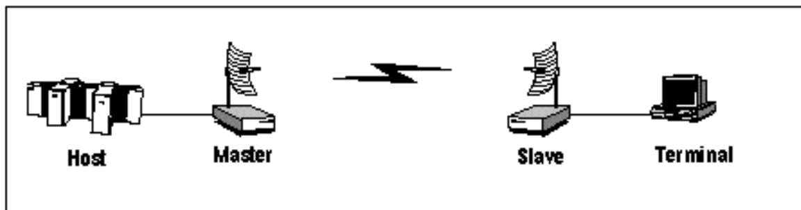
Figure 1-2 Point-to-Point Application Showing Master/Slave Configuration
