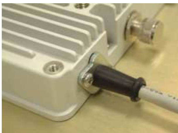
Figure 2-7: Cable connection to Outdoor Unit
