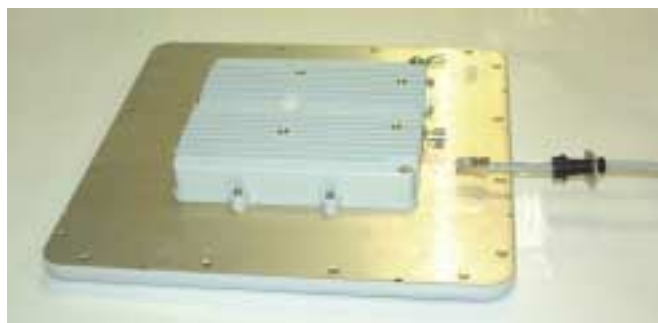
Figure 2-6: Cable insertion to Outdoor Unit.
