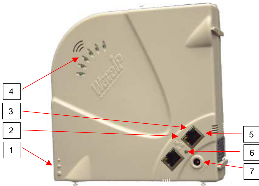
Figure 3-1: Description of Self Install GigAccess™ OFDM 900Q RSU
