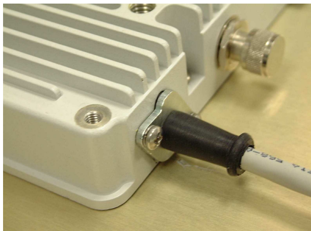
Figure 2-8: Cable connection to Outdoor Unit
