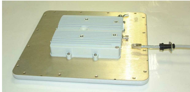
Figure 2-7: Cable insertion to Outdoor Unit.
