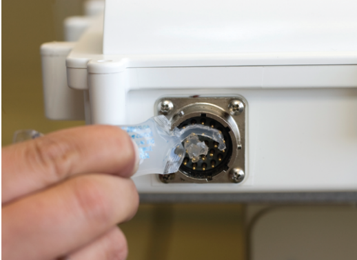
Figure 1.5 – Applying Silicon Dielectric Compound
