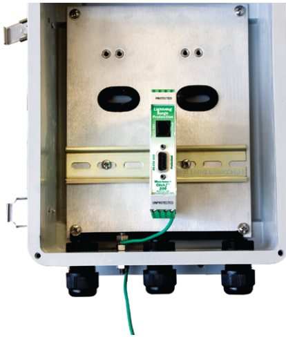
Figure 2.4 – Earth Ground Connections
