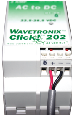
Figure 2.7 - Wiring DC Power Out of the Click! 201/202
