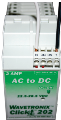
Figure 2.6 – Wiring AC Power into the Click! 201/202
