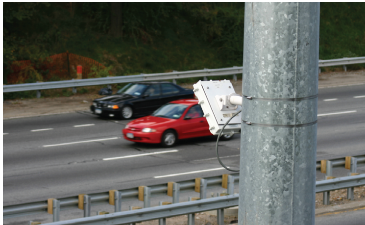
Figure 1.4 – Aiming the SmartSensor
