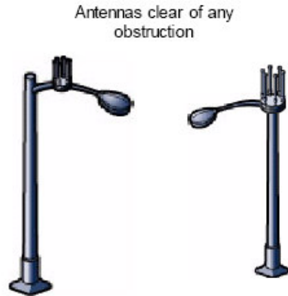
Figure 4.2 Example Mounting Locations on a Streetlight
