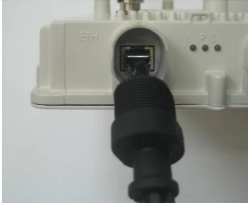
Figure 4.11 Connecting PoE cable
