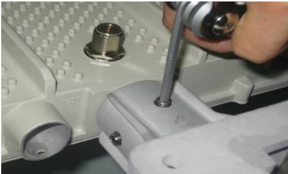
Figure 4.5 Attaching the WBS-2400/5800 to the pole bracket
