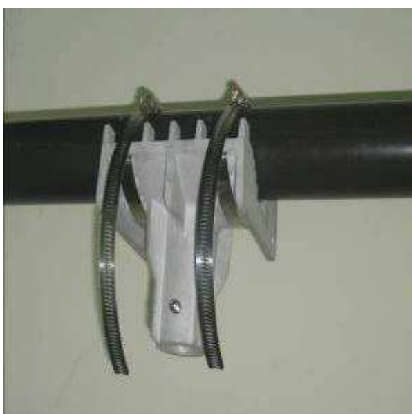
Figure 4.2 Using Special Hose Clamps & Screwing the Clamps
