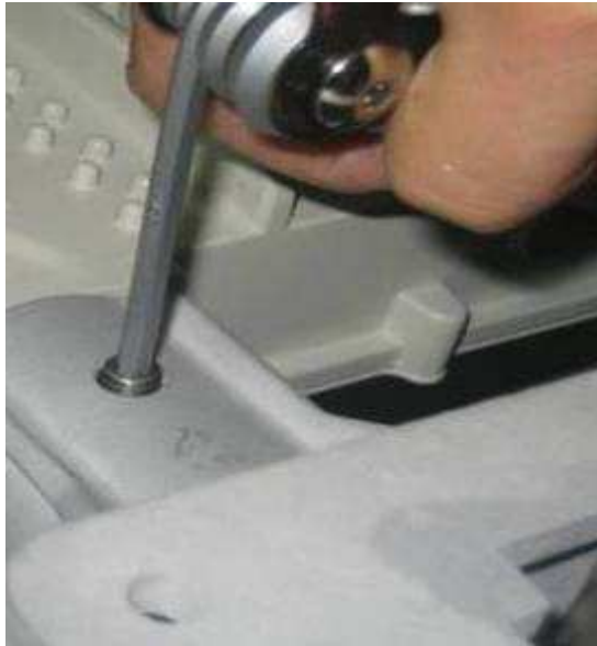
Figure 4.3 Attaching the WBS-2400/5800 to the pole bracket
