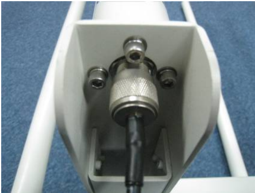
Figure 4.11 Connecting straight N-Type connector to the antenna
