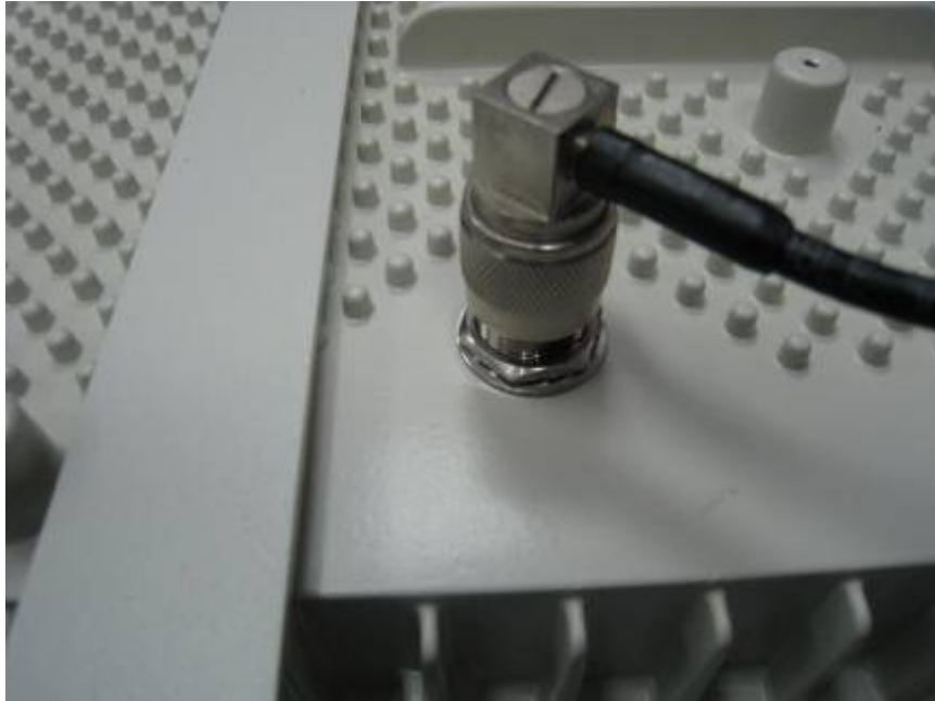
Figure 4.12 Connecting right angle N-Type connector to the antenna
