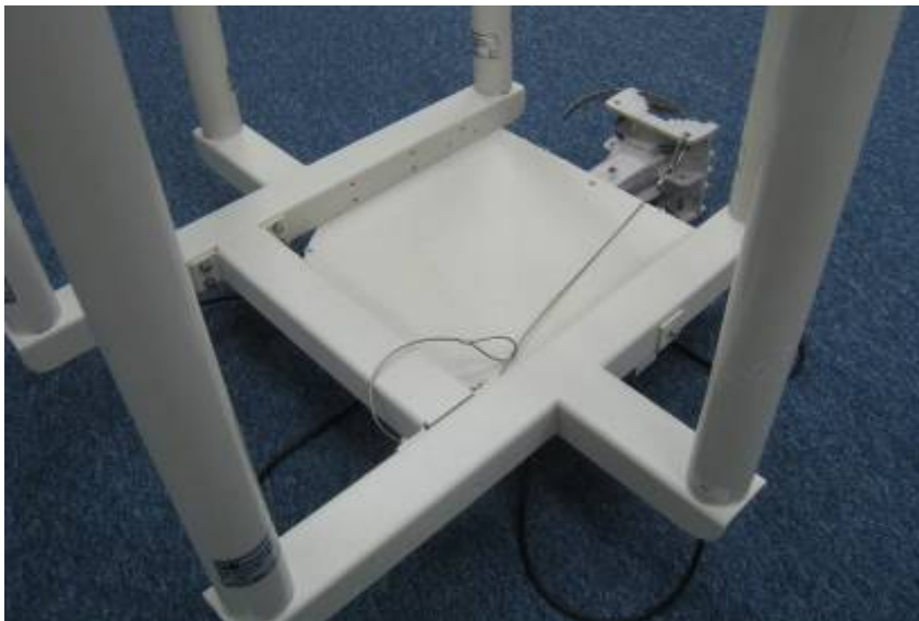
Figure 4.5 Attached Safety Cable
