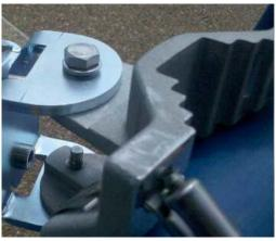
2. Slide the steel bands into the appropriate side slots of the post clamp.
